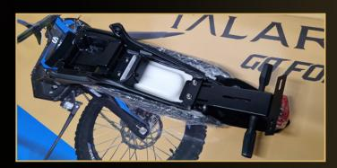
INSTALL TAIL TIDY TO SUBFRAME USING 2 X 10MM NUTS - ENSURE TAIL TIDY IS SAT LEVEL WITH THE SEAT AND FAIRING - ENSURE TAIL TIDY IS SAT LEVEL WITH THE SEAT AND FAIRING
