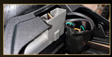
DISCONNECT & REMOVE THE BATTERY - EXPOSE REAR LIGHT CLUSTER SHROUD DISCONNECT ALL 5 CONNECTORS \* PLEASE NOTE ORANGE WIRE IS FOR LH INDICATOR AND BLUE WIRE IS FOR RH\*
